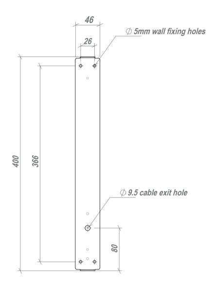
Backplates can be rotated 180 degrees- to allow cable exit to be positioned at top if required.
